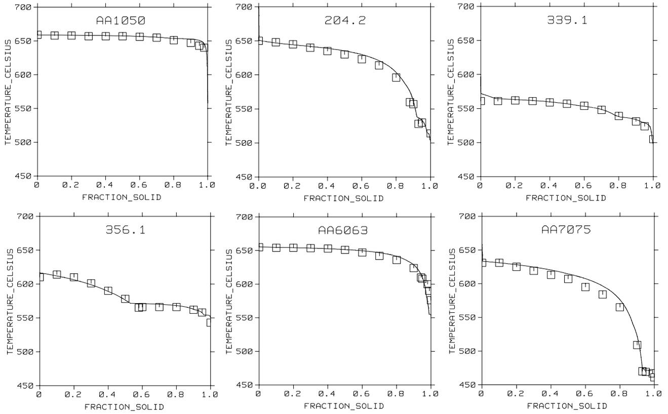
Figure 1. Fraction solid vs. temperature plots for various Al-alloys calculated under 'Scheil' conditions with experimental results ( $\square$ ) of Backerud et al [22] shown for comparison.
