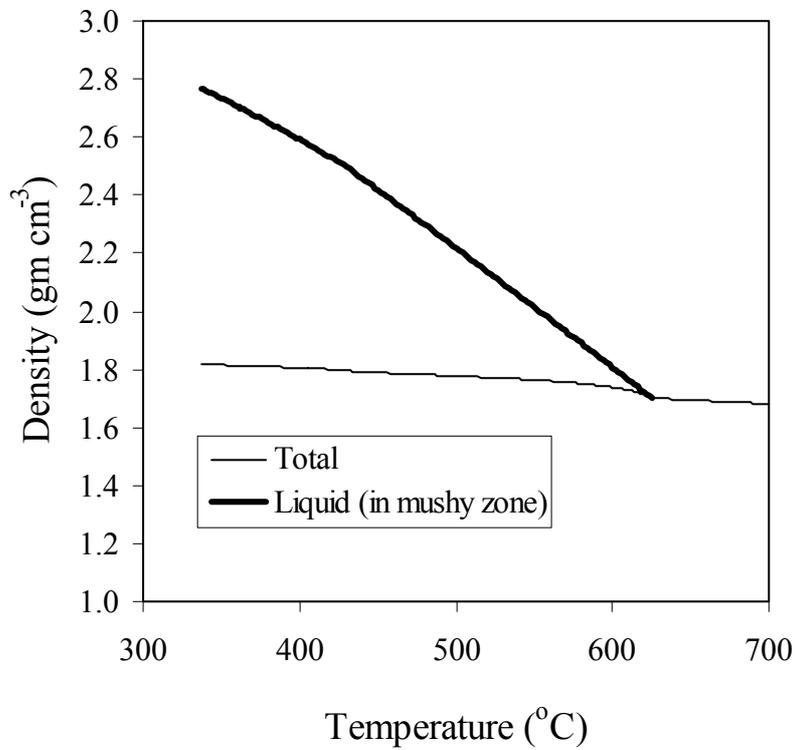
Figure 9. Calculated density of a ZMC711 Mg-alloy during solidification. Bold line shows density of the liquid in the mushy zone
