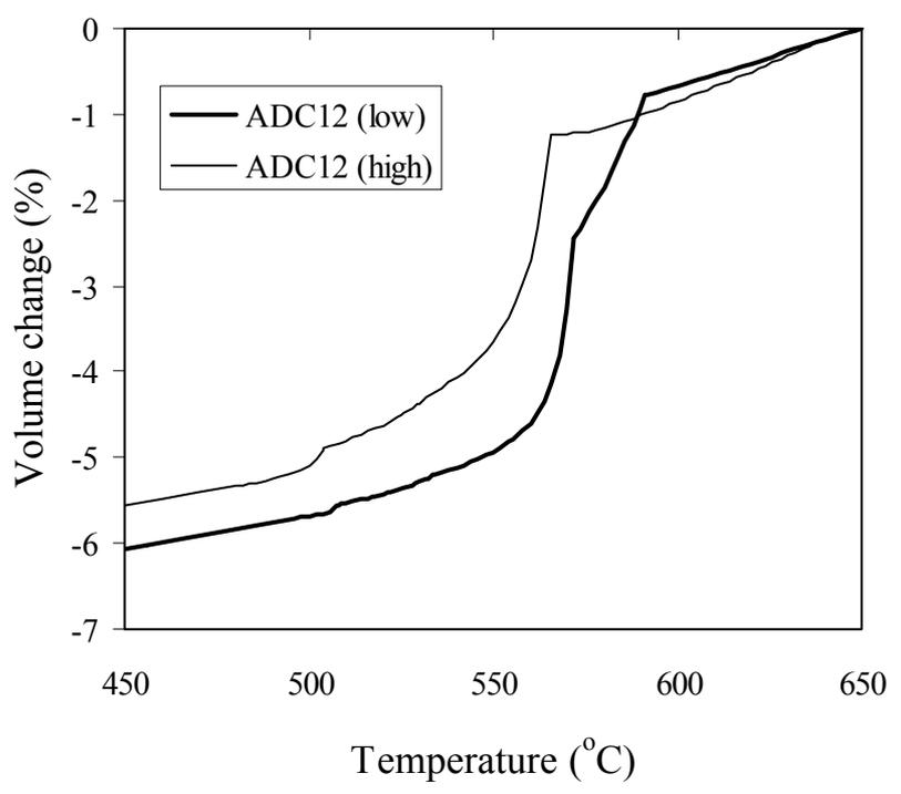
Figure 5. Calculated volume change vs. temperature plots of two ADC12 Al-alloys.
