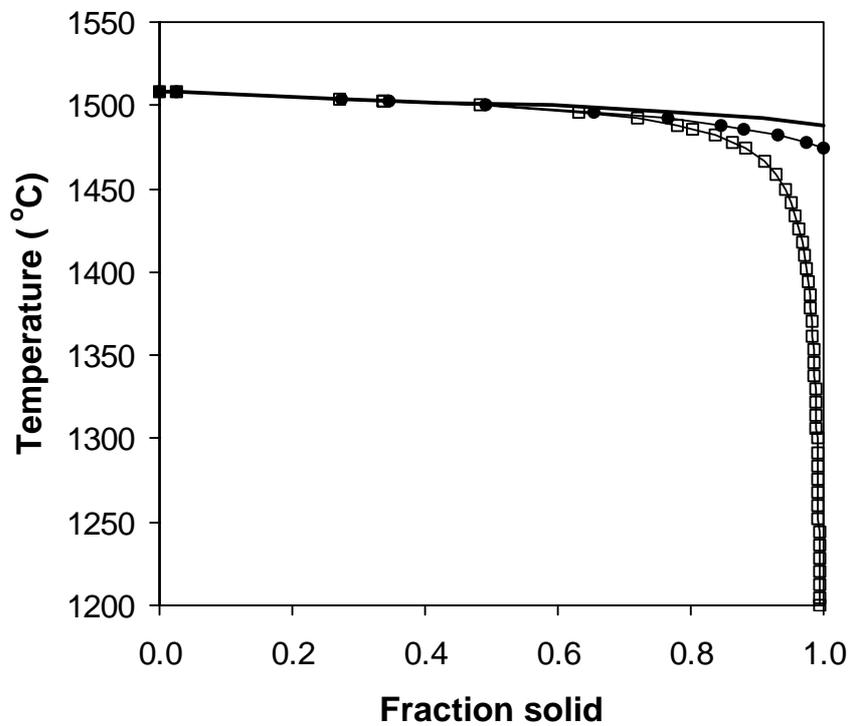
Figure 3. Fraction solid vs. temperature curves for solidification of a 3310 steel calculated under (—) equilibrium, ( $\square$ ) SG and ( $\bullet$ ) SGM conditions [15].
