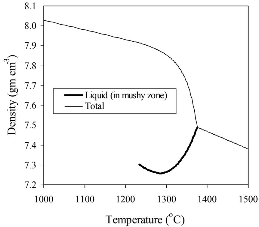
Figure 8. Calculated density of a SRR99 single crystal superalloy during solidification [18]. Bold line shows density of the liquid in the mushy zone
