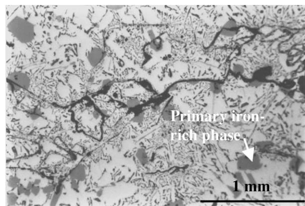
Figure 3 Optical micrograph of Alloy 2 casting sedimented at  $600^\circ\text{C}$  for 4 h showing oxide films and primary  $\alpha\text{-Al(FeMn)Si}$  particles at the base of the casting.
