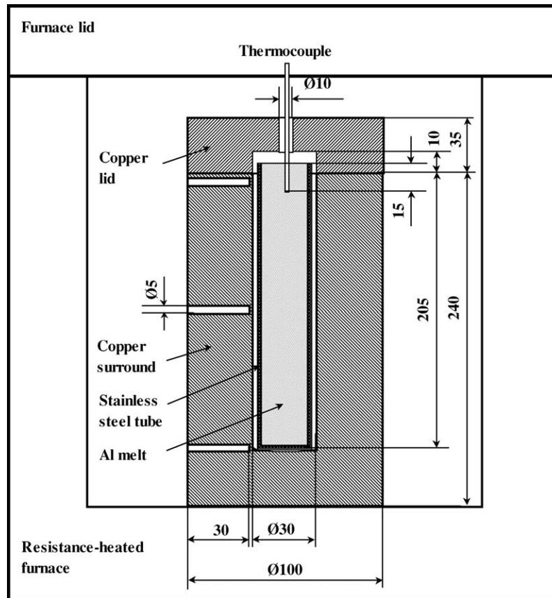
Figure 1 Experimental set-up used for convention-free sedimentation. Dimensions shown are in mm.
