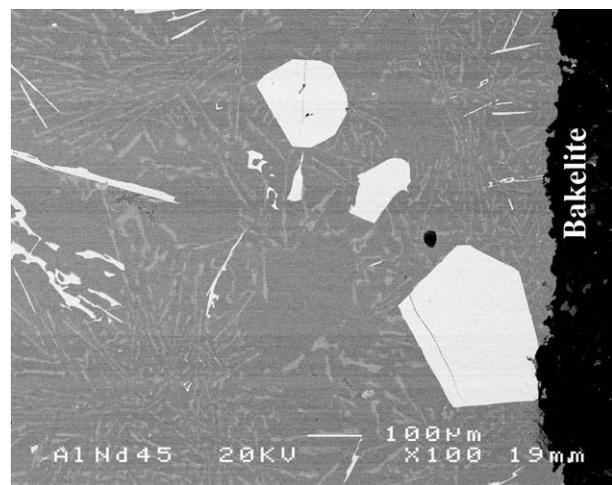
Figure 2 Back-scattered electron image taken at 70 mm from the base of Alloy 2 casting sedimented at  $600^\circ\text{C}$  for 4 h showing primary  $\alpha\text{-Al(FeMn)Si}$  particles on or near the stainless steel mould wall.
