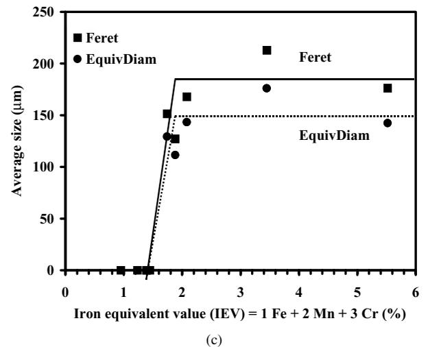
Figure 7 (a) Equivalent circle diameter and (b) feret diameter quantifying the effect of original Fe and Mn contents on the sizes of primary  $\alpha$ -Al(FeMn)Si particles, and (c) average equivalent circle and feret diameters as a function of the original IEV.
